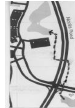
Figure 5 The dashed line shows the path of the drainage system under Nicholls Road
