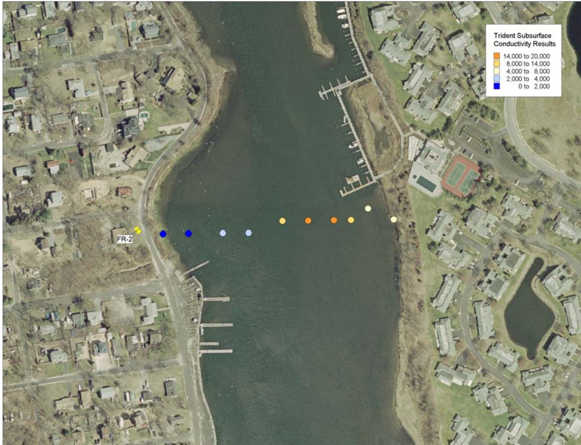
Figure 3-3. Site map showing Trident conductivity results for transects FR-2 (conductivity values are in \mu\text{S}/\text{cm} ).
