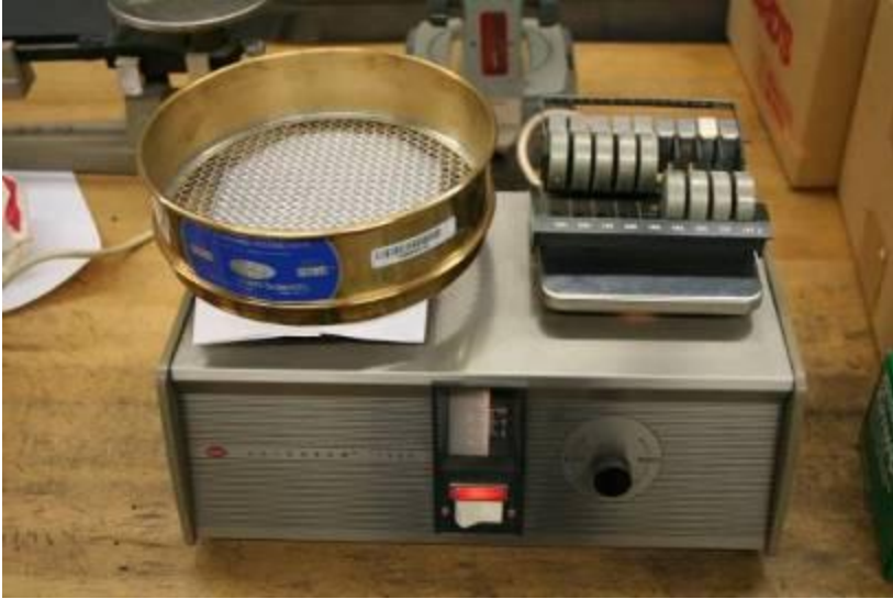
Figure 2.2 Weigh and record sieves to 0.01 gram
