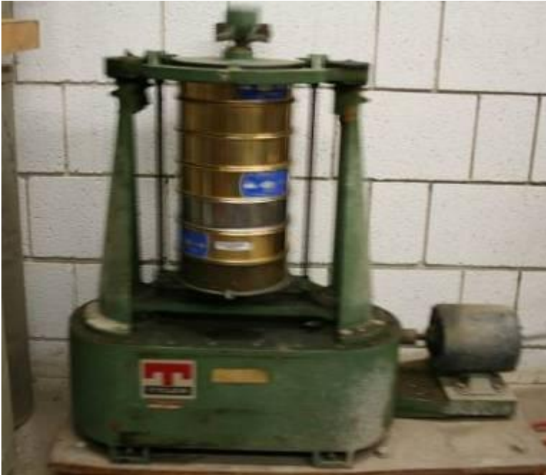
Figure 2.4 Shake the Sieve Set with Sample in the sieve shaker.
