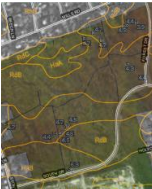
Figure 8 – pH of surface soil using distilled water in contact with the soil for one day on a soil map with overlay of the digital elevation model in Fig. 6
